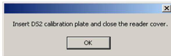
Insert the same Cal plate into the upper carrier, close the cover, and click “OK”. The reader will proceed to scan the plate. When finished, the following will be displayed.
