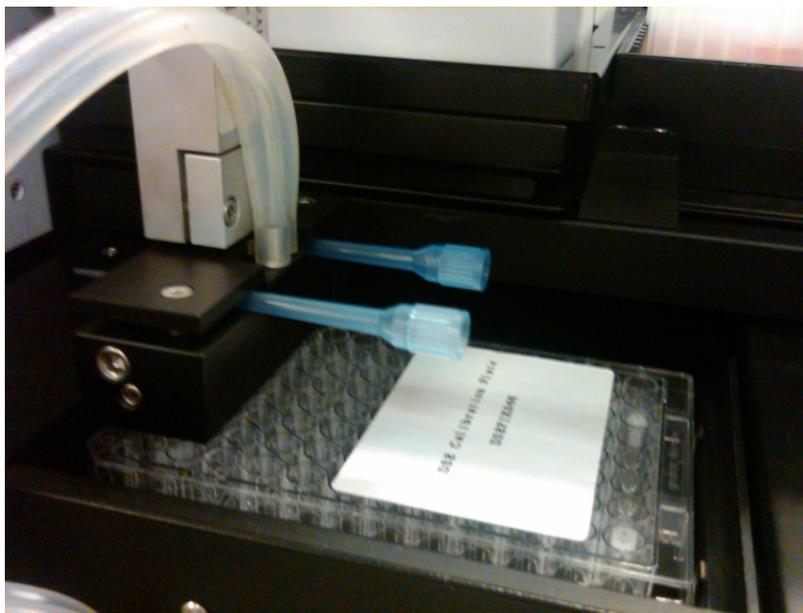
2. Please note: The plate carriers will move if you apply too much force while performing the calibration. Be gentle when inserting the aspiration pins into the white well inserts in the plate, taking care not to move the plate carrier around. If the plate carrier is moved, calibration values will be incorrect.
