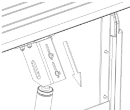
To **decrease** the Gas Spring Force position the Sliding Bracket further up the adjustment slots
