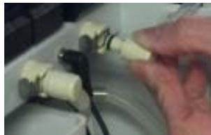
**WARNING:** The waste bottle trap must be connected to the **RIGHT** waste bottle tubing. Failure to do so will result in improper operation of the waste bottle trap.
